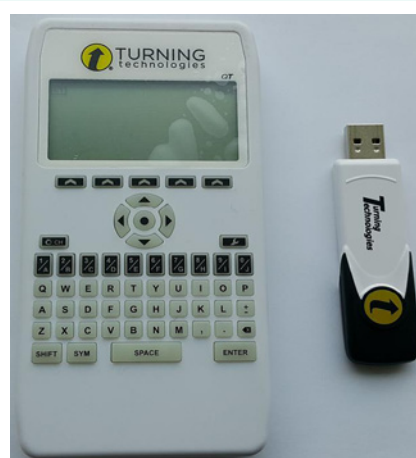
Figure 1: Turning technology clickers with radio frequency receiver.
